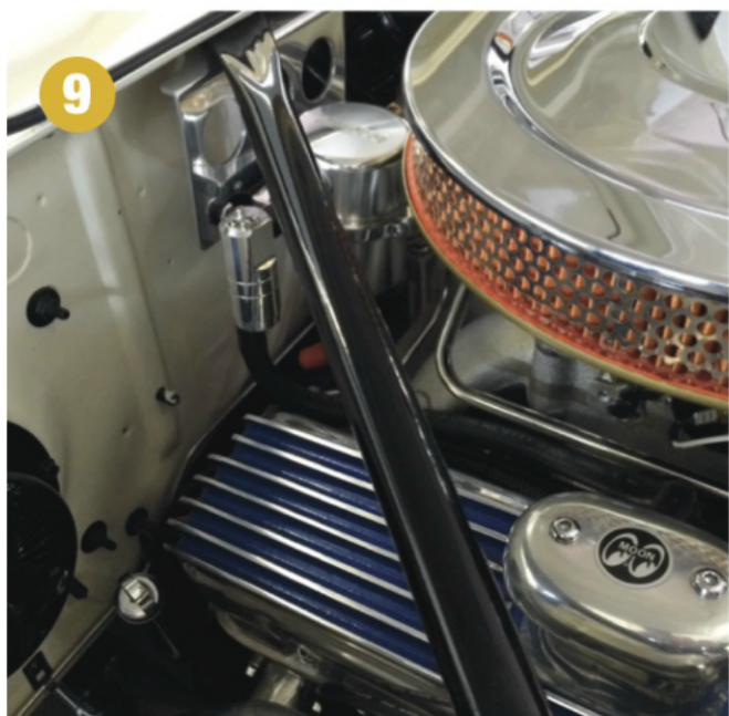
Figure 9: DF-17 Dual Flow PCV Valve with Inline adaptor installed used in conjunction with oil air separator
