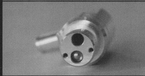
There are two check balls in the valve, one which is spring loaded (bottom) and regulates the flow under cruising conditions. What looks as a black hole (top) is where the idle circuit check ball lives. If you're really curious about what's inside, we strongly recommend looking at the cut-aways on the M/E Wagner website instead of taking the valve apart. Although, it is serviceable and rebuildable.
