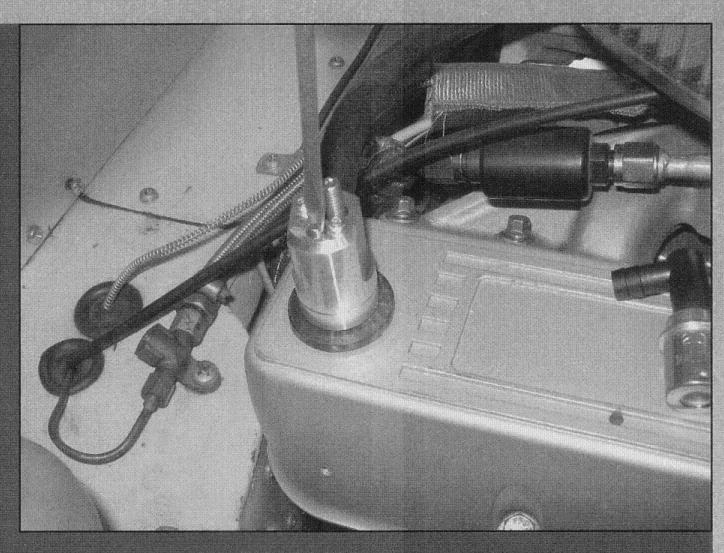
And there you have it. Properly adjusted, now the blowby will get sucked back into the carb and burnt off, your idle mixture screws should be functional again (if the old valve let too much air through) and, well, life is good.
