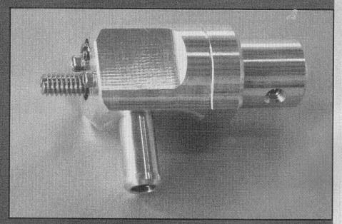
anyway? It's supposed to suck out just the right amount of fumes from the crank case, ridding it of moisture and acidic vapors, which keeps the interior of a motor clean and helps the oil stay cleaner. Clean oil is good, right? Also, a PCV valve that doesn't match the motor can render the carb un-tuneable.
