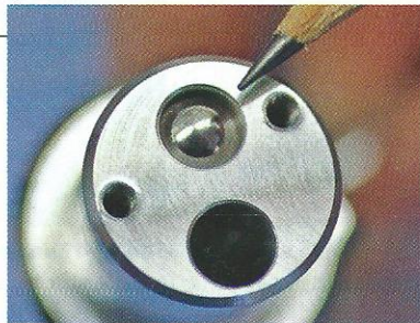
The single plunger (OE-style) is replaced with two balls for flow control.
