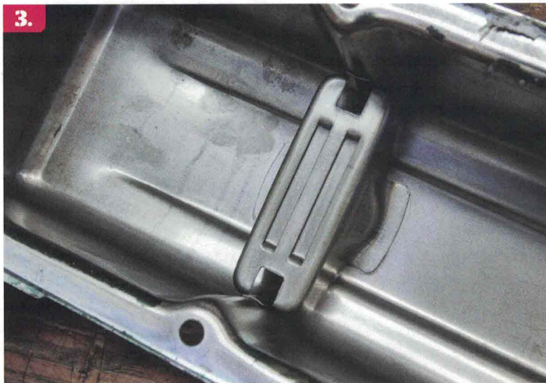
3. This is a typical vapor separator inside a small-block Chevy valve cover. Tight clearances sometimes do not do an adequate job of separating oil from the vapor because liquid oil can travel along these surfaces and be ingested into the PCV valve. Wagner has a video on his website that illustrates this.
