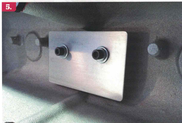
5. HOMEMADE BARRIER Matt Wagner's experiments for creating an efficient oil separator inside a valve cover created this simple barrier. It is designed so its sides do not touch the valve cover and that it stands off from the top of the valve cover by at least 3/4 inch. This slows the movement of the oil and air, allowing the oil to separate. If the clearances are too close, the air movement is fast enough to carry the oil with it into the PCV valve.
