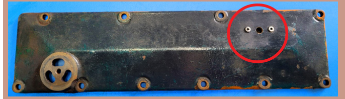
1929-1931 Valve Cover (side plate) with a drilled and tapped hole and crude riveted aluminum baffle installed inside. This hole is now my new fresh air inlet (J).
