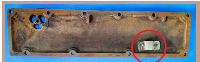
1929-1931 Valve Cover (side plate) with a drilled and tapped hole and crude riveted aluminum baffle installed inside. This hole is now my new fresh air inlet (J).
