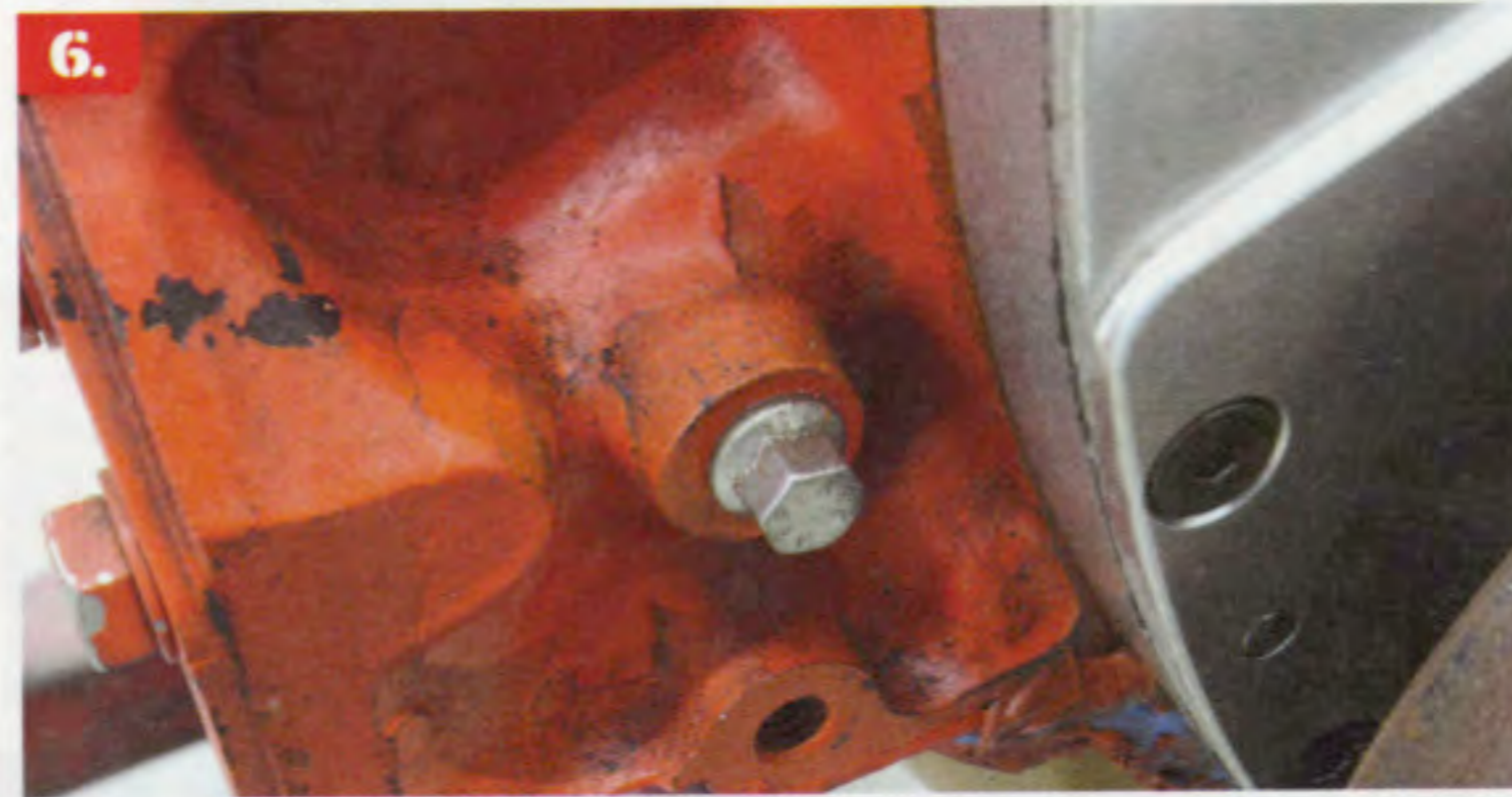
6. Most two-piece rear main seal blocks feature this tapped, 3/8-inch bolt boss in the front near the fuel pump. This hole is drilled into the channel for the fuel pump pushrod. If this short, 3/8-inch bolt is omitted, it becomes an obvious leak channel. Make sure the bolt is short enough to not contact the fuel pump pushrod.
