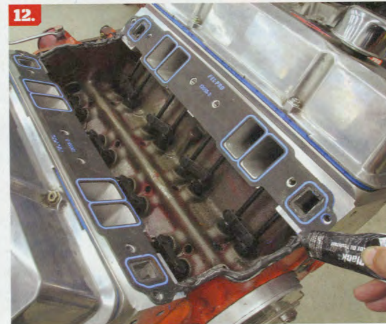
12. A line of RTV roughly ¼ inch in diameter is usually sufficient to seal between the china wall's front and rear and the intake manifold. Placing a small dab of RTV under the little tabs at the bottom corner of each intake gasket will help seal the corners.
