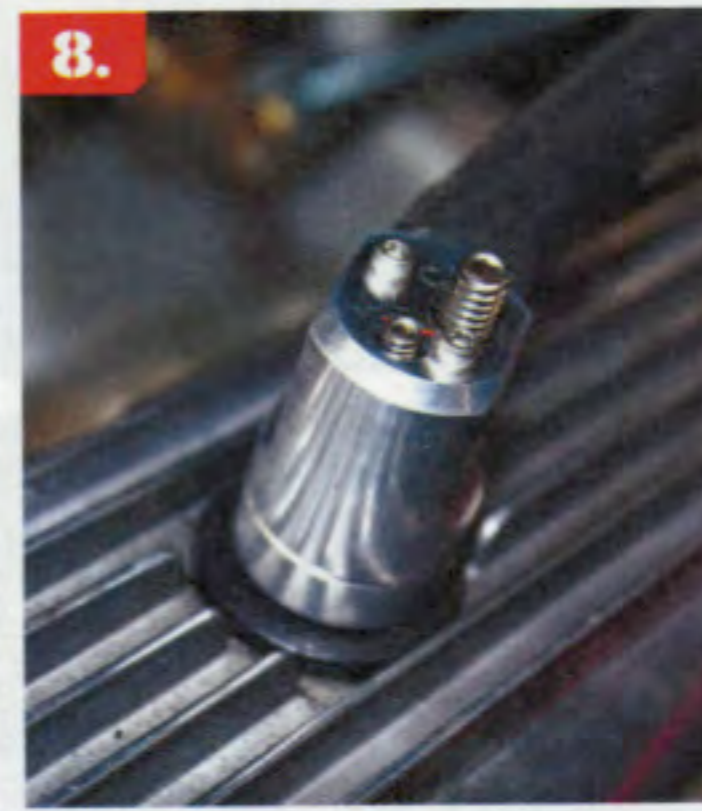
7-8. One of the best ways to minimize leaks is to reduce the inevitable pressure in the crankcase by using an M/E Wagner billet, adjustable, dual-circuit PCV valve. This valve will reduce crankcase pressure, which will immediately reduce the potential for oil leaks. This valve is best combined with a vapor separator canister because the valve flows so well that it can more easily pull oil out of the engine if the valve cover is not properly baffled.
