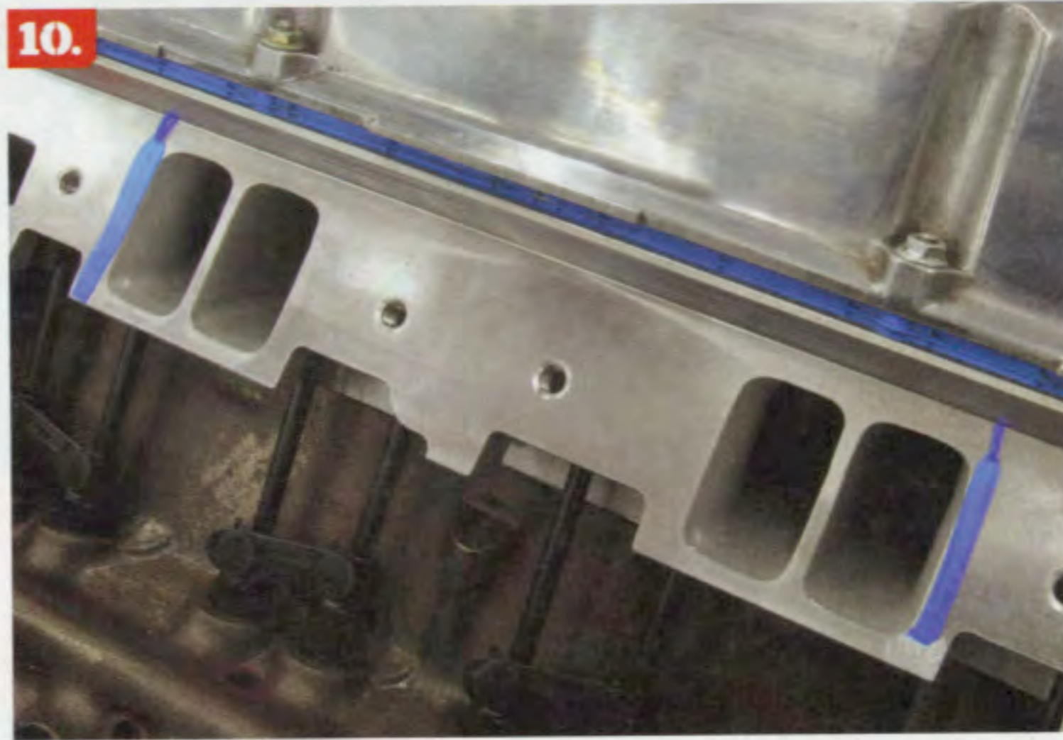
10. If your engine is using oil but not leaking, it might be pulling oil from the bottom of the intake gasket because the intake gasket sealing surface is not parallel with the cylinder head. This test uses 0.100-inch-diameter wax string placed on all four corners of the intake ports as shown without gaskets. Bolt the intake on and then remove and look at how much the string is squeezed. If the string is wider at the top than the bottom, the two surfaces may not be parallel. Repairing this requires machining the intake manifold to produce parallel planes.
